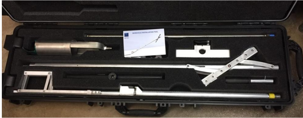
Figure 3.6 Teros Borehole Installation Tool kit with an auger.
