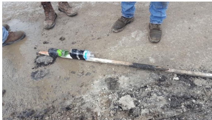
Figure 3.14 Simple water-bailing tool formed to discard excess water in boreholes.
